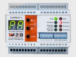
This is a quick guide to DIP Switch Setup on the SC10 when building a starter panel. These are suggestions for a starter panel for common dewatering pumps. The starter is primarily for Snore control, but optionally with support for floats.
